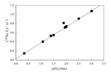
**FIG.1.** Measured <sup>129</sup>Xe  $T_1^{-1}$  as a function of O<sub>2</sub> partial pressure for samples of a few bar of Xe and O<sub>2</sub>. The fitted line is a regression analysis omitting the one outlying point and was used to derive the empirical relation between <sup>129</sup>Xe  $T_1$  and  $pO_2$ . Error bars are the same size or smaller than the data symbols.
